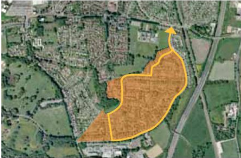
Figure 5-2 Poorly connected development with a single entrance/exit for all modes
